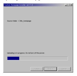
The following page will appear after a while. The camera will be restarted automatically in two minutes, and storing to the built-in flash memory is completed.
